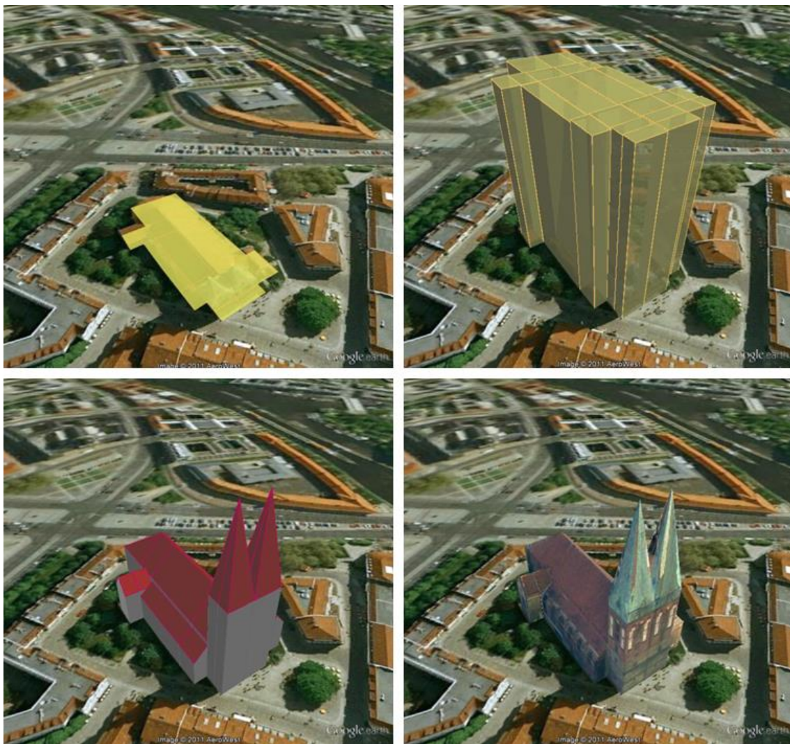
Figure 73: The same building displayed as (top down and left to right) footprint, extruded, geometry, COLLADA
