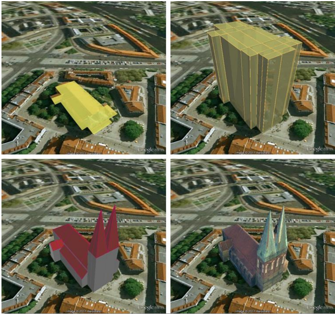
Fig. 13: The same building displayed as (top down and left to right) footprint, extruded, geometry, COLLADA.
