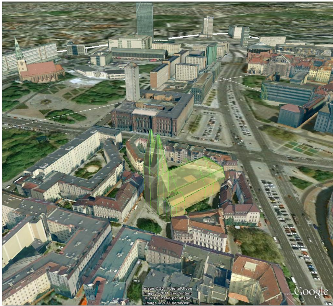
Fig. 16: Object exported in the COLLADA display form being highlighted on mouseOver.
